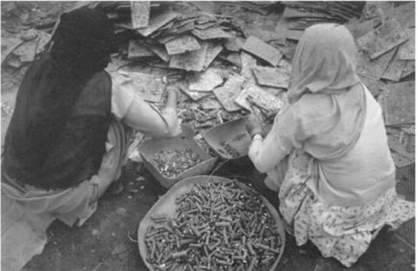
PHOTO 21.3. Women using simple tools to remove semiconductor chips, transistors, capacitors, and other items from electronics circuit boards at e-waste facility in India. Courtesy of Toxics Link, India.
